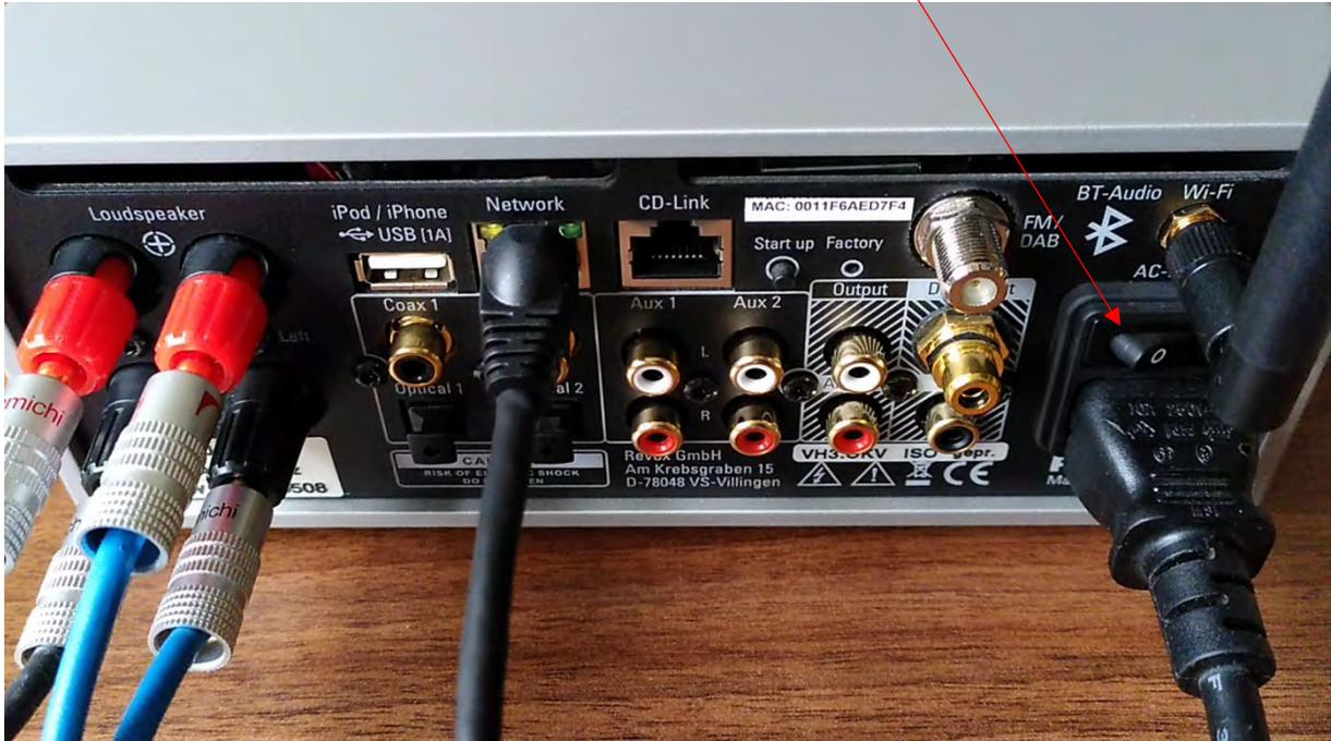
3. In order for the JOY S119 to obtain an IP address of your network of the DHCP range, press the Start up button on the back. This sets the JOY S119 to DHCP and obtains a new IP address.
