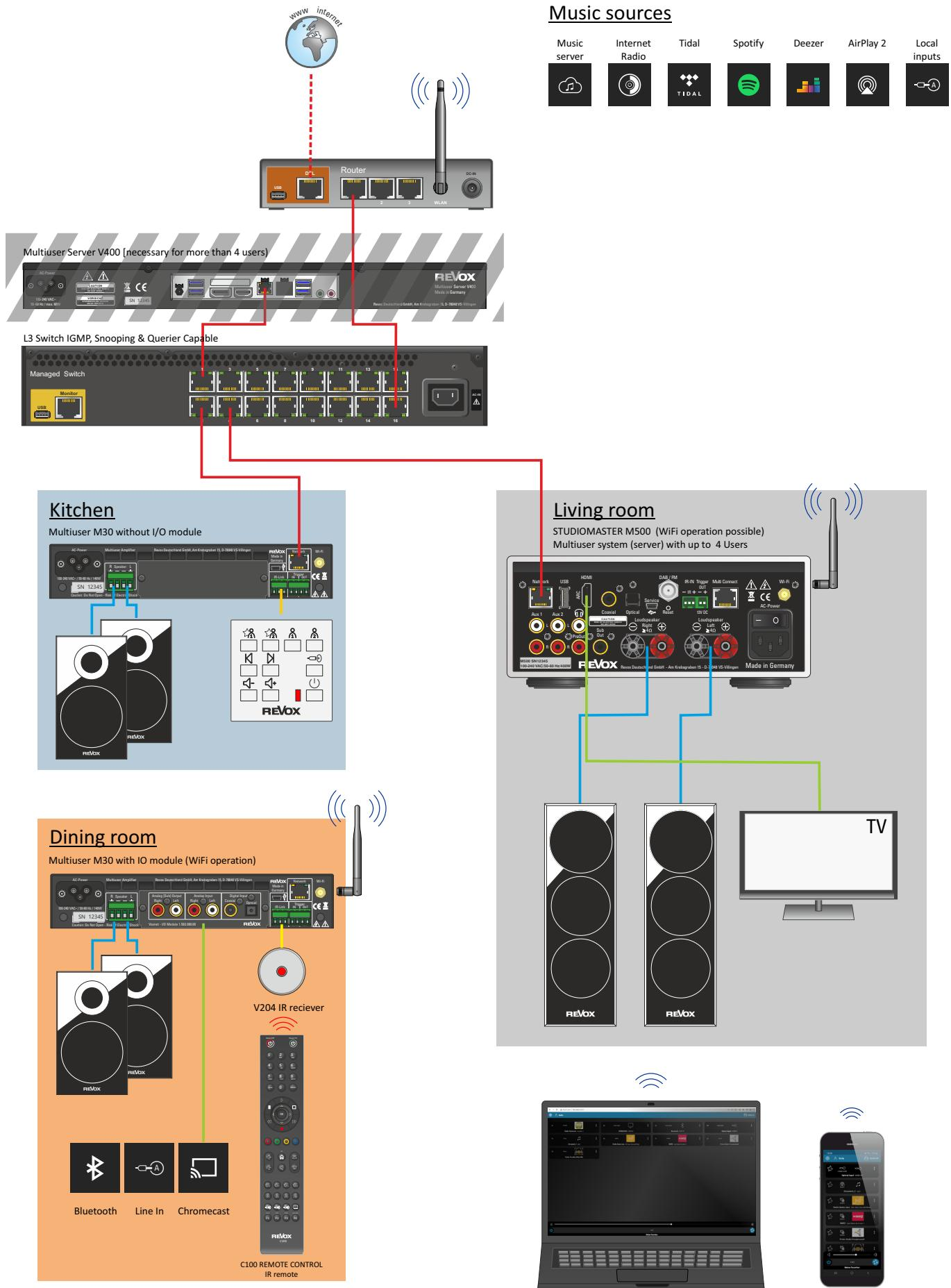
Revox Multiuser System - Schematic diagram without KNX
