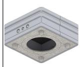
Ceiling installation housing consisting of EPS base body with glued-in OSB rear wall cover and OSB front with cut-out for installation in concrete ceilings.
