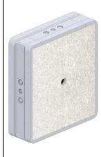
Universal installation housing Wallboxx, designed for masonry and concrete walls. The Wallboxx enables professional installation of built-in speakers. Front and rear panels are made of OSB and integrate seamlessly into the workflow for easy further processing of the wall surface. The surrounding base body made of EPS is low in resonance and has sound-insulating properties. The loudspeaker opening has to be made by a self-cut-out.
