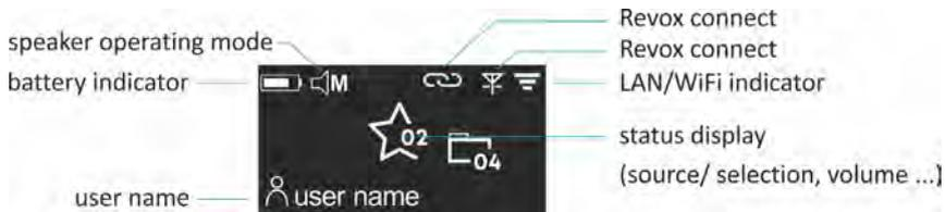
**Revox Connect** is a connection routine that uses Bluetooth to establish an initial connection between the A200 and your mobile device. Using the Revox Multiuser app, the A200 can now be informed of the WLAN network with its key (password) via a Bluetooth connection.
